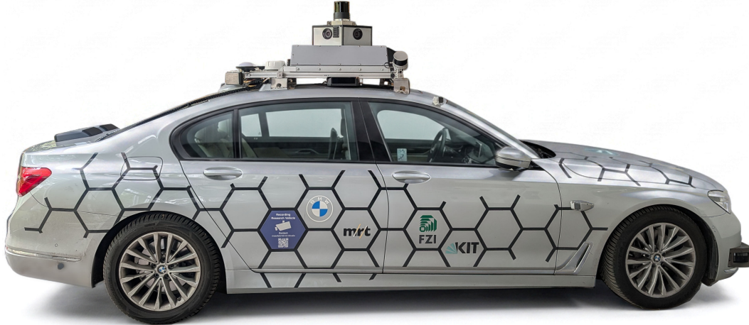
Figure 10: The KITScenes recording vehicle with the sensor setup as roofmount.
